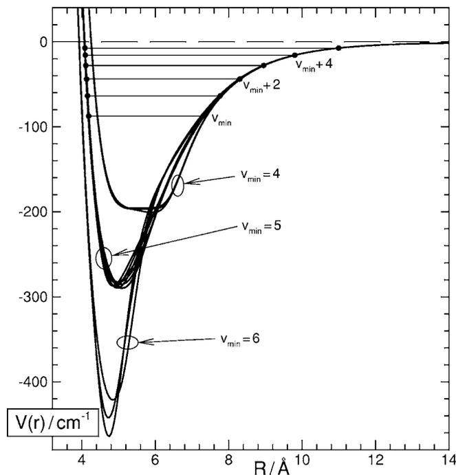
FIG. 5. Four fitted potentials for  $v_{\min}=4$ , eight for  $v_{\min}=5$ , and three for  $v_{\min}=6$ , all of which account for all of the available data within the estimated experimental uncertainties (standard errors  $\leq 0.005 \text{ cm}^{-1}$ ).
