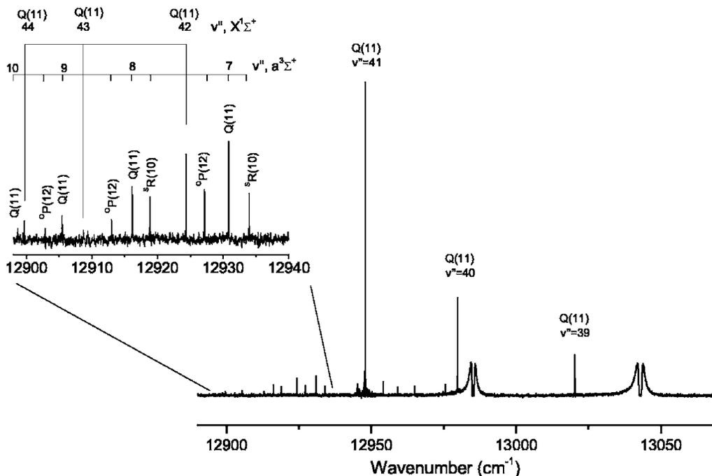
FIG. 2. Fluorescence from  $v'=20, J'=11f$  of  $B^1\Pi$ , with  $Q$  lines seen in the  $B-X$  system, and  $Q$  lines with strong  $^5R, ^0P$  satellites to  $a^3\Sigma^+$ . The potassium  $D$  lines at  $12\,985.17$  and  $13\,042.88\text{ cm}^{-1}$  are self-absorbed.
