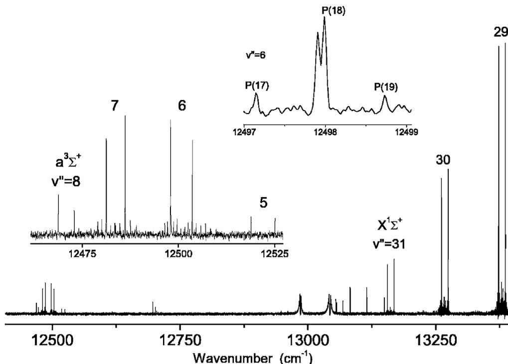
FIG. 4. FT emission spectrum showing well-separated transitions to the  $a^3\Sigma^+$  and  $X^1\Sigma^+$  states of  $\text{K}^6\text{Li}$  obtained following excitation to  $B^1\Pi$  ( $v'=10$ ,  $J'=17$ ,  $e$  parity). Rotational relaxation patterns are seen in both the singlet and triplet systems; they originate from different upper states.
