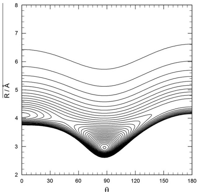
**Fig. 1.** Contour plot of the fitted He–N<sub>2</sub>O potential energy surface (for  $v_3 = 0$ ) as a function of  $R$  and  $\theta$ . The angles  $\theta = 0$  and  $\pi$ , respectively, correspond to the oxygen and nitrogen ends of the impurity. The contours descend from 0 to  $-62 \text{ cm}^{-1}$  with an interval of  $2 \text{ cm}^{-1}$ .
