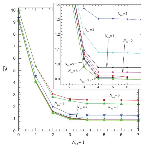
**Fig. 9.** Test of convergence of the fits as a function of  $N_{\Omega}$  for different choices of the order  $N_{\text{na}}$  of the polynomial function used to represent the centrifugal BOB correction function.
