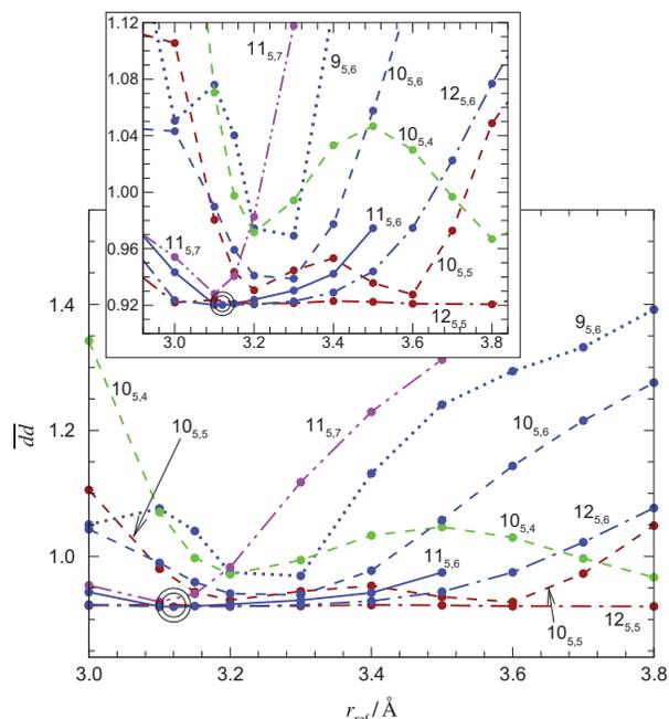
**Fig. 5.** Variation of the quality of fit  $\overline{dd}$  with the radial variable expansion centre  $r_{\text{ref}}$  for a number of different MLR models for the  $X^1\Sigma_g^+$  state of  $\text{Br}_2$ . The labels for the various cases are  $N_{p,q}$ , where  $N \equiv N_\beta$ .
