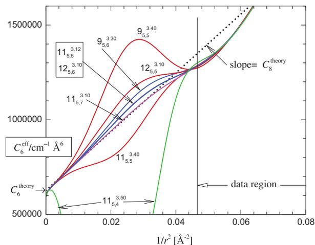
**Fig. 7.** Test of the long-range extrapolation behaviour of a number of fitted MLR models for the  $X^1\Sigma_g^+$  state of  $\text{Br}_2$ . The labels for the various cases are  $N_{p,q}$ , where  $N \equiv N_\beta$ .
