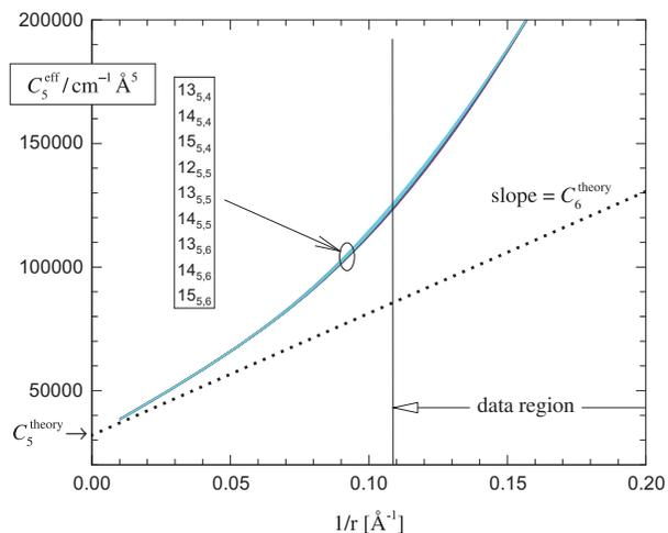
**Fig. 8.** Test of the long-range extrapolation behaviour of a number of fitted MLR models for the  $A^3\Pi_{1u}$  state of  $\text{Br}_2$ . The labels for the various cases are  $N_{p,q}^{\text{ref}}$ , where  $N \equiv N_{\beta}$ .
