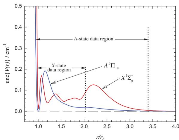
**Fig. 13.** Uncertainties in the final A- and X-state potential energy functions implied by the 95% confidence limit uncertainties in the potential function parameters yielded by the fit.
