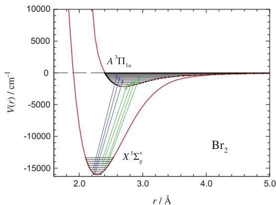
**Fig. 1.** Overview of the  $A^3\Pi_u-X^1\Sigma_g^+$  system of  $\text{Br}_2$  with representative magnetic rotation transitions [16] shown in blue and laser absorption transitions (present work) in green. (For interpretation of the references to colour in this figure legend, the reader is referred to the web version of this article.)
