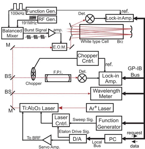
Fig. 2. Block diagram of the Ti:Sapphire ring laser spectrometer.
