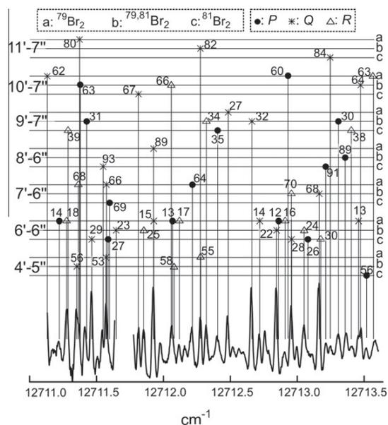
Fig. 3. Recorder trace of Br<sub>2</sub> absorption lines in the 12711.0–12713.5 cm<sup>-1</sup> region.
