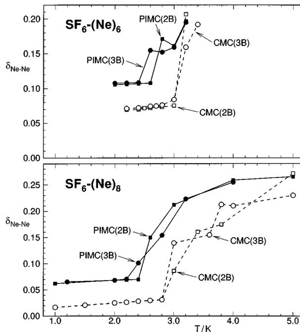
FIG. 9. Melting curve plots for two monolayer isomers of  $SF_6-(Ne)_n$  obtained using classical (open points, dashed curves) and quantum PIMC (solid points, solid curves) simulations which either included (round points, labeled “3B”) or neglected (square points, labeled “2B”) the three-body ATM interactions.
