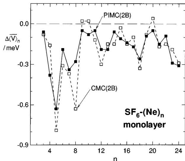
FIG. 8. Changes in the average potential energy per Ne solvent atom in monolayer  $\text{SF}_6-(\text{Ne})_n$  clusters at 1 K, as additional Ne atoms are added to the system.
