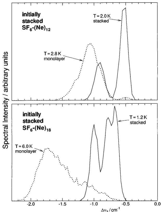
FIG. 12. Predicted shifted spectra of the  $\nu_3$  band of  $\text{SF}_6$  yielded by quantum PIMC simulations of initially-stacked isomers of  $\text{SF}_6-(\text{Ne})_{12}$  and  $\text{SF}_6-(\text{Ne})_{18}$ . In both cases, at the higher temperature the system collapses to the monolayer form during the simulation run.
