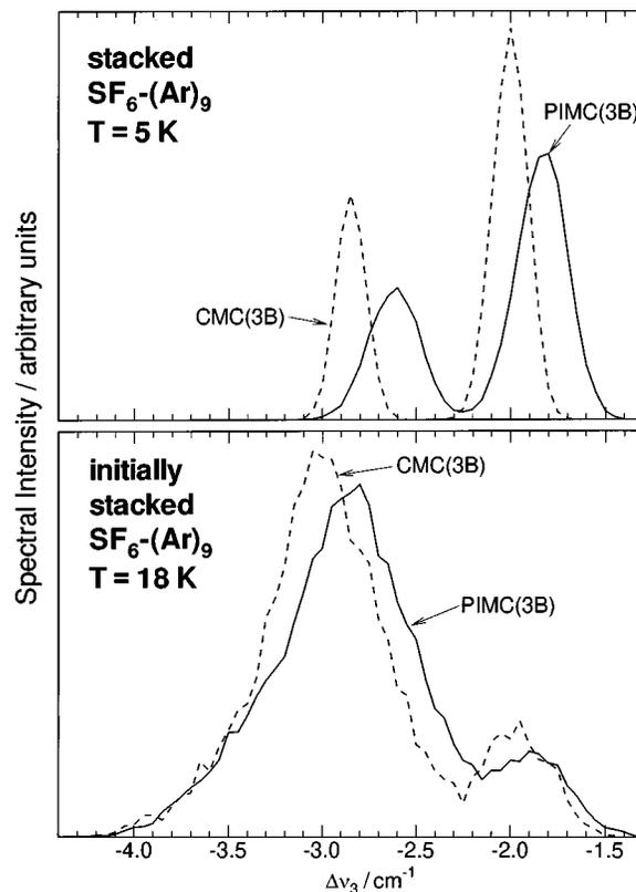
FIG. 7. Predicted shifted spectra of the  $\nu_3$  band of  $\text{SF}_6$  yielded by classical (dashed curves) and quantum (solid curves) simulations for the initially stacked 6+3 isomer “9F” of  $\text{SF}_6-(\text{Ar})_9$ .
